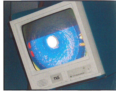
Closed Circuit TV: Color monitor with camera mounted in the Roto-Max ® Automatic cabinet for ease of process viewing.
