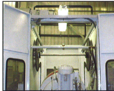
Environmental Package: Noise cover and internal lighting for the Roto-Max ® Automatic.
