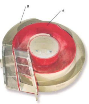
Heat can be supplied to Channel B by use of heat lamp assemblies or a hot water jacket around the bowl.
