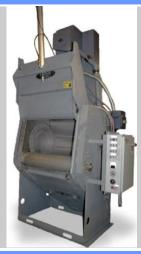
(1) 15 Hp Direct Drive Blast Wheel 6 cu. ft. or 800 lb. Load Capacity Mill Drive Motor with Current Sensor for Mill Jam Protection Reversing Mill \* Mill Bypass Cast Barrelhead Liners Low Level Sensor & Indicator Light
