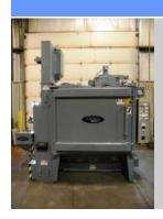
(1) 15 Hp Direct Drive Blast Wheel 5,000 lb. Load Capacity Dial Blast Cycle Timer Hour Meter, Amp Meter Work Table Accessible by Overhead Hoist Work dimensions: 48" diameter x 28" high
