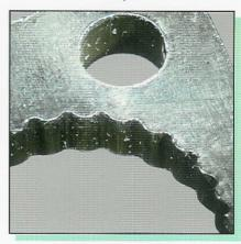
Edge Break With Planetary Head 2000/Hr.
