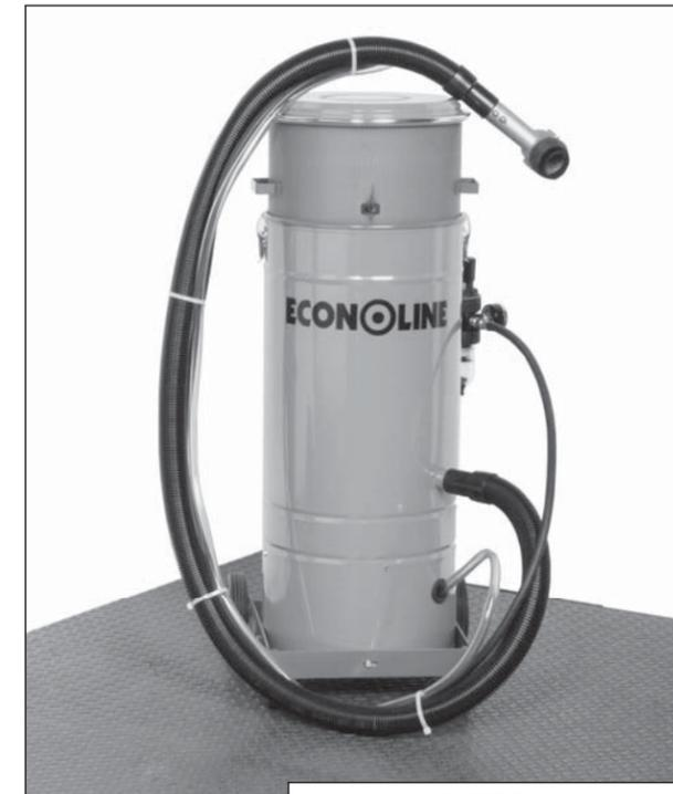
The Econoline ESB 007 Spot Blast unit is a portable, dust free solution to your blasting needs. Low abrasive consumption recycles abrasive media separate from dust and debris. Includes a standard 12 CFM trigger gun, regulator and gauge, water filter, recycling head and a .5 micron cartridge filter. This unit weighs just 55 lbs when empty, and with a 1" blast pattern, it's perfect for small jobs and touch ups.
