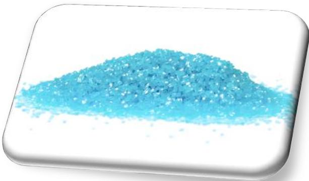
Polycarbonate-based cryogenic blasting medium for cryogenic deflashing of rubber parts.
