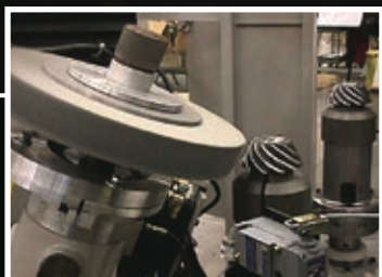
Scotch-Brite® Wheel producing edge radius on bevel gear.
