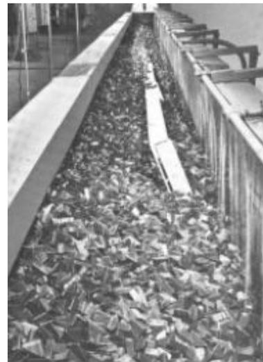
**Channel created by coupling multiple Vibratrons**
